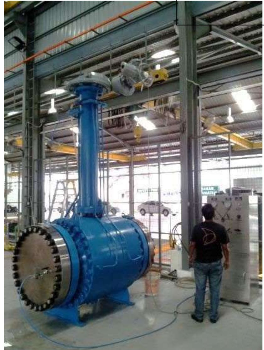
Assembly of one of the motorised actuated valves (30" diameter) in our Shah Alam facility.
